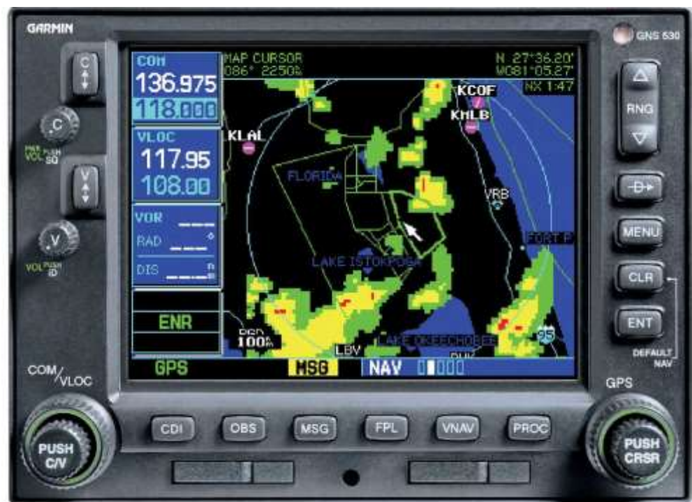
Figure 4 - Garmin GNS 530 WX navigation computer
